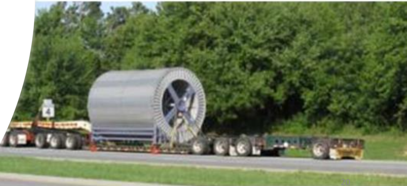
Figure 10-Oversized Reel Transport, 4,724 feet of 230kV Cable
